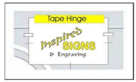
Lift the graphic back on the hinge to that it lies flat and carefully peel the packing paper. Carefully flip the graphic back on its hinge and hold it away from the substrate.
